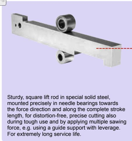
Sturdy, square lift rod in special solid steel, mounted precisely in needle bearings towards the force direction and along the complete stroke length, for distortion-free, precise cutting also during tough use and by applying multiple sawing force, e.g. using a guide support with leverage. For extremely long service life.
