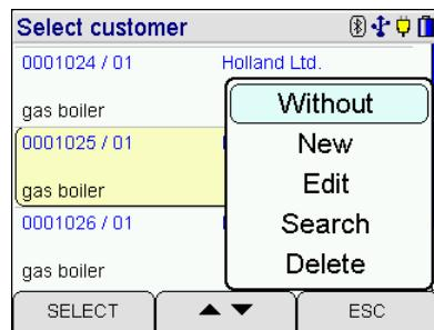
A previously selected customer number is shown in the result display with (REF). The customer number can be changed before storing.
