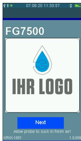
During the first 30 seconds, the device conducts a stabilization and a system check. This is shown by the progress bar below the time display and by the green square in the header. The measuring function cannot be used during this time. Administrative functions can be used during this time.
