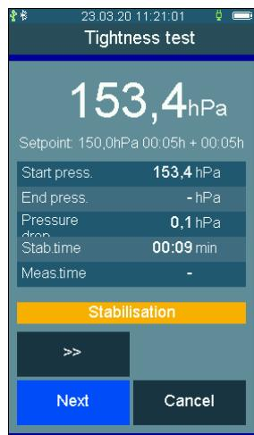
Measurement: The pressure pattern as well as the starting, end and differential pressure are recorded during the measurement period. The selected measurement period can be shortened using **“Quit”**.
