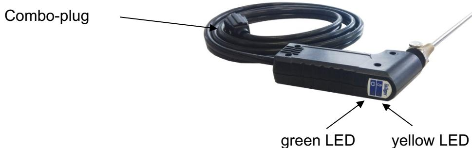
The green LED indicates the exhaust probe being ready for measurement.
