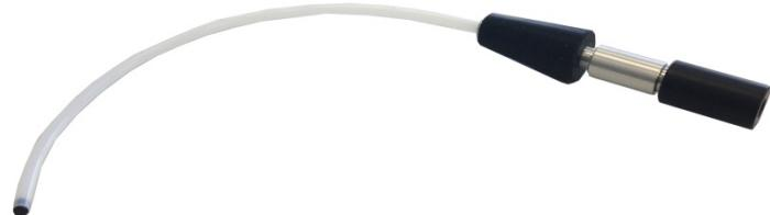
The annular adapter is inserted on the probe tube of the exhaust probe for the measurement and locked into place.
