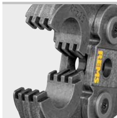
Pressing tongs with teeth prevent formation of burr on the pressfitting. Patent EP 2 027 971
