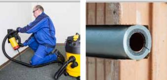
Full contact support plate during the entire chasing/cutting process for guided plunge-in of the diamondcutting discs, dust-free, safe working and easy, even feed.
