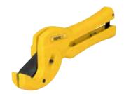
Robust quality tool for clean, fast cutting of pipes in one cut. Stable magnesium version. For one-hand operation.
