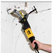
sawing also during extreme load conditions, e.g. sawing of steel pipe. Adjustable mechanisms with a great variety of parts and a reduced system stability do not withstand the high feed forward pressure and the heavy-duty requirements of forceful cutting of steel pipes, particularly when a guide support with leverage is being used.
